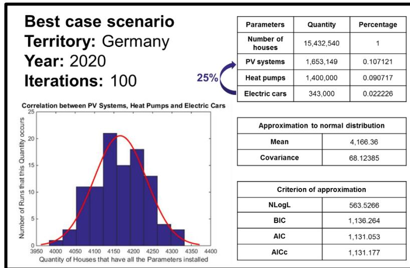
**Fig. 6.** Results for a German best-case scenario in 2020 with a dependency of 25% from electric cars to PV systems
