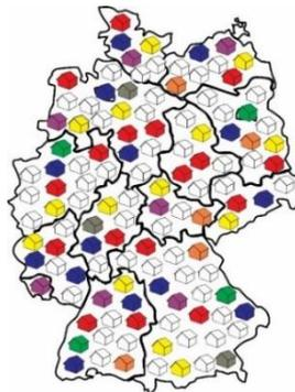
**Fig. 4.** Step 4: When other element is distributed, for example heat pumps (blue), it is possible to collect the number of all the houses that have potential for HEM systems. They are houses with an electric car and a heat pump (green), an electric car and a PV system (orange), a heat pump and a PV system (purple) and an electric car, a PV system and a heat pump (grey).
